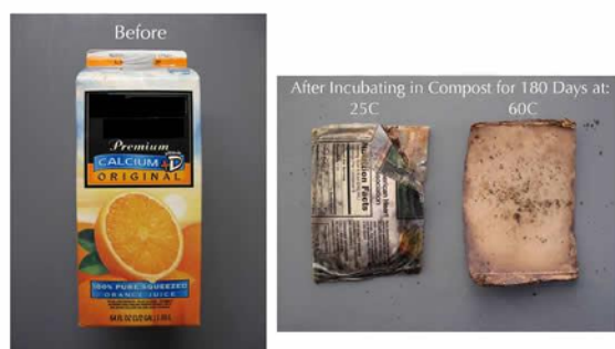
FIGURE 2. MICRO-PLASTIC PARTICLES WERE RELEASED FROM ALL PLASTIC-COATED PAPER PRODUCTS SUCH AS THIS PAPER ORANGE JUICE CARTON, SHOWN BEFORE AND AFTER TESTING.
