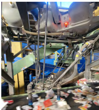
Robot removing containers and plastic film from the paper stream.
