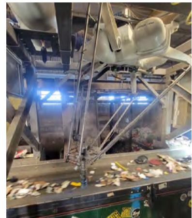
Robot separating recyclables from the residual stream.
