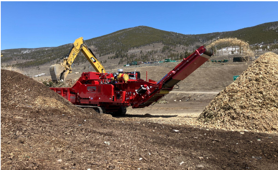
The RotoChopper chipping wood at the SCRAP. Photo: Bill Schenk, SCRAP
