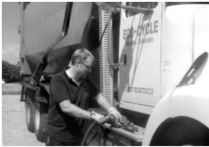
Eco-Cycle driver Rodger Keep fuels up the first Eco-Cycle truck to run on a biodiesel fuel blend. Biodiesel is made from soybeans and other vegetable oils and is a cleaner-burning, domestically-produced alternative to petroleum-based diesel fuel.
